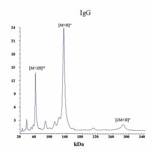
Profiler's high mass range capability is demonstrated by this mass spectrum of 1 pmole of Immunoglobulin G antibody. The dimer (2M+H)+ ions is clearly visible at 300 KDa.
